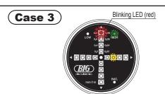
①The levelling value of one of the axes exceeds 0.08 after turning ON the power. The LED (red) is blinking.
