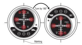
②Rotate the device by 180° using as reference the markings on the reference surface.
