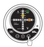
(6) Push the MODE switch to change to the HIGH (7) Adjust the level in order to turn on the LED (blue) of the central position.
