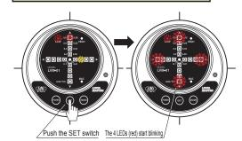
①Push the "SET" switch after 10 seconds. The 4 external LEDs (red) start blinking.
