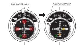
③Push again the "SET" switch after 10 seconds. The buzzer will emit a "Beep" to notify the completion of the "zero adjustment".
