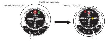
(5) Adjust the level in order to turn on the LED (blue) of the central position in the LOW mode. When the LED (blue) turns on, the inclination is within 0.1.
