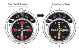
③Push again the "SET" switch after 10 seconds. The buzzer will emit a "Beep" to notify the completion of the "zero adjustment".
