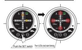
①Push the "SET" switch after 10 seconds. The 4 external LEDs (red) start blinking.
